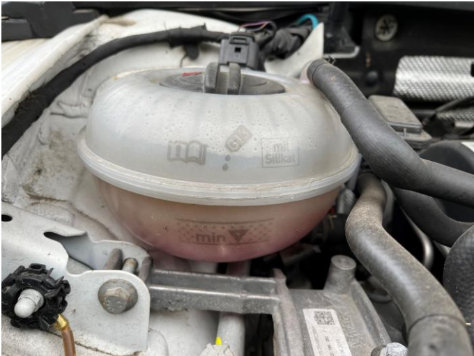
Check the tightness of the expansion tank and the cap.
