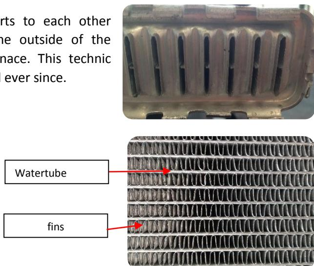
Since a few years car manufactures have switched from Alu/Plastic Brazed system (plastic tanks and aluminum cores) to Alu/Alu system this to provide better cooling and reduce the chance of leaks to an absolute minimum.
