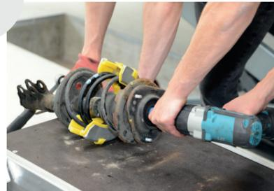
6. In the next step, compress the suspension strut using a spring compressor. Once the spring is sufficiently compressed by the spring compressor, the nut can be loosened from the top strut mounting, and the top strut mounting can be removed together with the spring cap.
