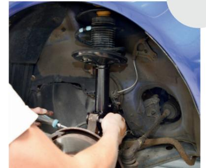
11. Finally, tighten the nuts on the top strut mounting and shock absorber fully once more. Important: it is imperative to perform an axle alignment after replacing a shock absorber, a coil spring or a top strut mounting like the ones that are also available in the Jakoparts range!
