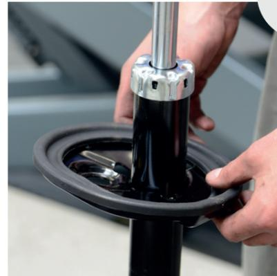
8. Ideally replace all rubber components and install these on the new shock absorber from Herth+Buss. Important: when mounting the spring cap on the suspension strut, ensure that the guide mount sits on top of the one on the shock absorber.
