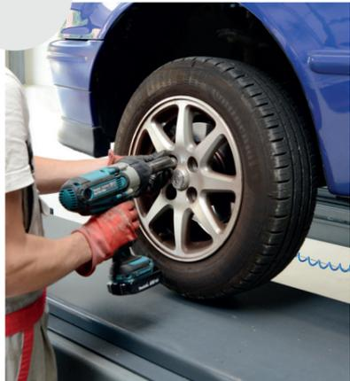
2. Raise the vehicle and remove the wheel.
