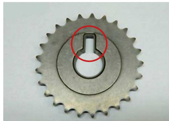
Fig. 2 Sprocket with key slot
