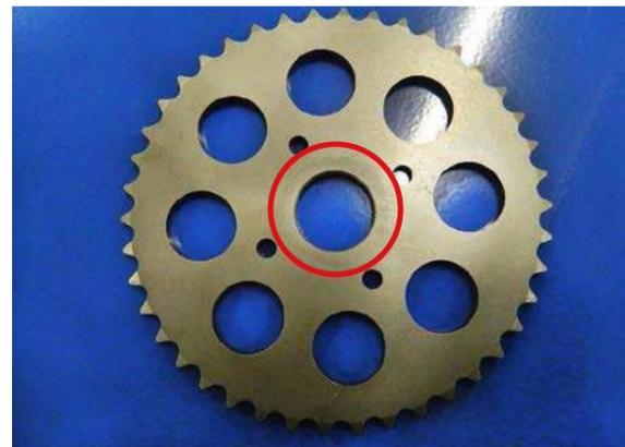
Fig. 1 Sprocket without key slot
