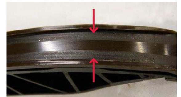
Excessive wear on plastic part of the guide. Inadequate lubrication has caused the chain to elongate and collide with the guides.
