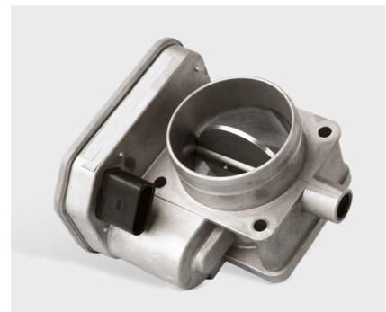
In diesel vehicles, the difference in pressure between the exhaust and intake side is not sufficient for the high exhaust gas recirculation rates. As a result "regulating throttles" are placed in the intake manifold to generate the vacuum required.
