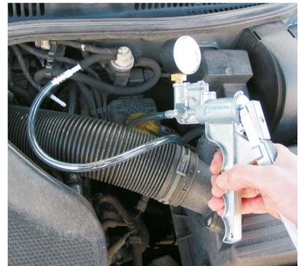
Whether pneumatic EGR valves or a pressure transducer like here – the function can easily be checked using a vacuum hand pump.
