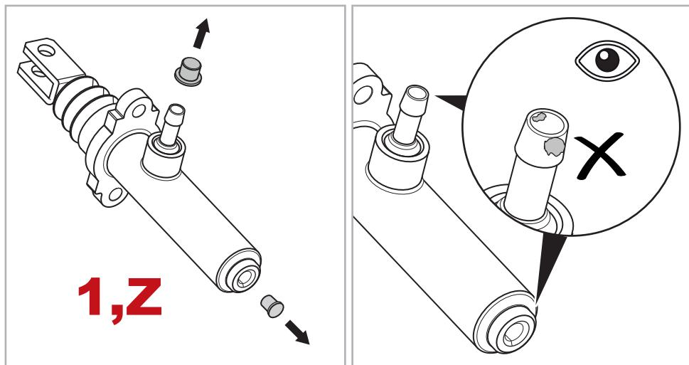
**EN** Remove the protective caps from the new clutch cylinder and prevent dirt from entering the connectors. Dirt or corrosion inside the clutch cylinder leads to malfunctions (piston does not move smoothly or gets jammed).
