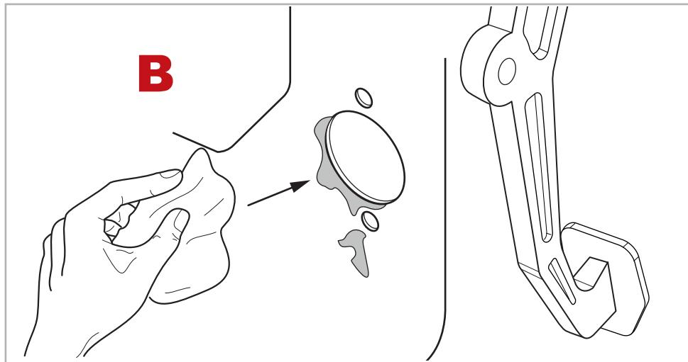
**EN** First of all, clean the assembly surface / contact surface of the clutch cylinder.
