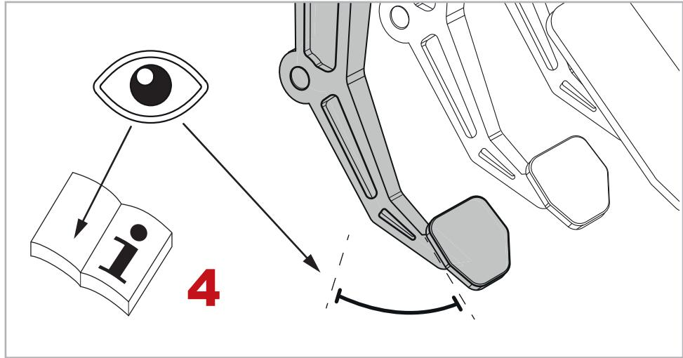
**EN** The actuation travel of the clutch pedal must be set according to the manufacturer's specifications. Also check the stop screw and/or the rubber buffer.
