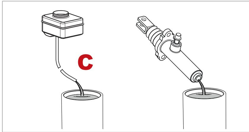
**EN** Remove any liquids from the reservoir and cylinder.
