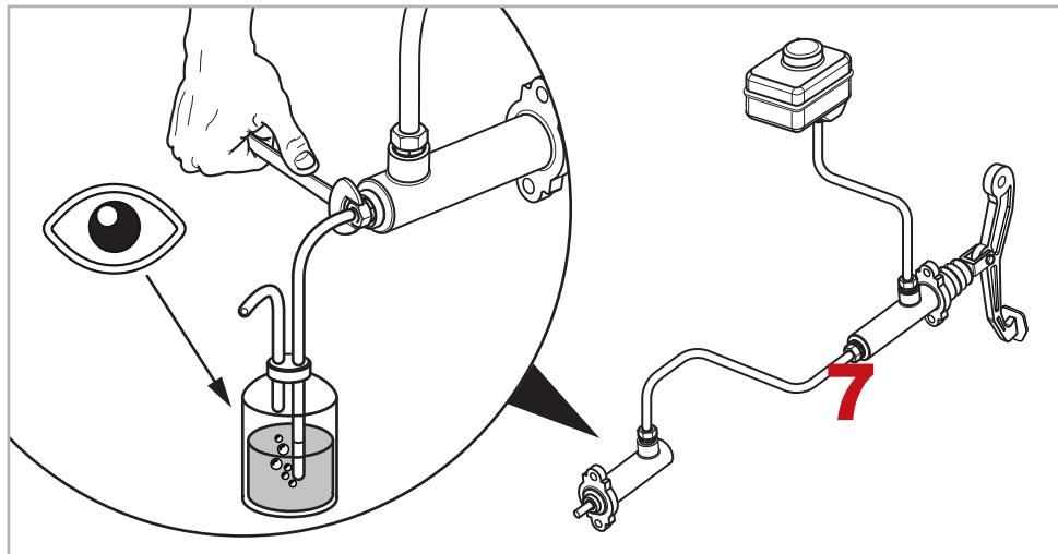
**EN** Vent the hydraulic circuit according to the manufacturer's specifications. Ensure a sufficient air supply.
