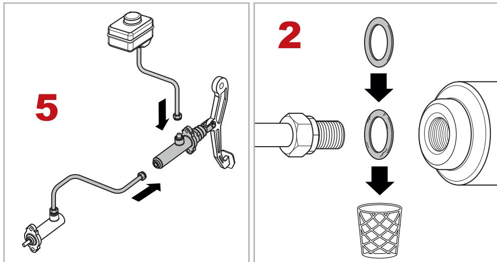
**EN** Connect the pneumatic and / or hydraulic hoses and pay attention to the correct connections. If required, use the new seal rings for mounting the pneumatic and / or hydraulic hoses to the clutch cylinder. Observe the tightening torques (Nm) specified by the vehicle manufacturer.
