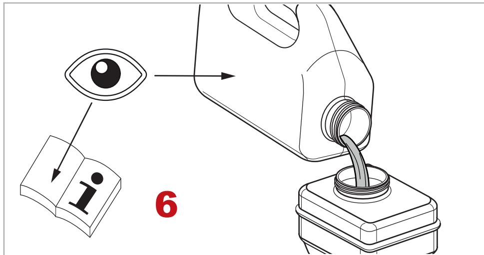
**EN** **Important:** Fill the reservoir with a sufficient amount of new (unused) supplies. Always use the supplies specified by the manufacturer in order to ensure the proper functioning of the clutch cylinder.
