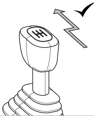
**EN** Take a test drive on your premises to check for smooth gear change. If the clutch cylinder reacts irregularly, with a delay, or does not react at all (the clutch cannot be actuated, does not disengage, slips or jumps), this may be due to the following:
