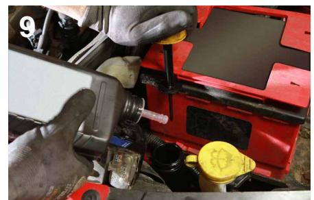
10. (Person 2) When the container is filled with oil, start the engine (idling only). Steer slightly from one side to the other, preventing complete deflection so that the pump does not build up the maximum pressure.
