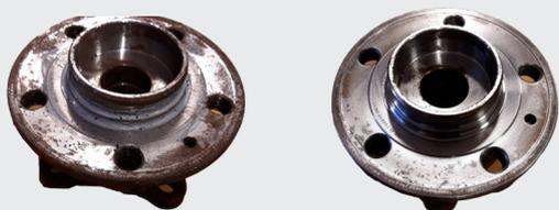
Clean the contact surfaces of the wheel hub to remove all depositions/corrosions.
