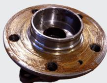
**DO NOT use grease/copper paste** on the contact surfaces between the wheel hub and the brake disc.
