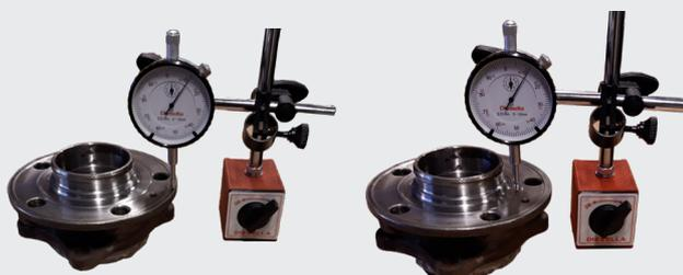
Check the contact surfaces of the wheel hub for deformations with a micrometer clock (Max. fling 0,03 mm.)
