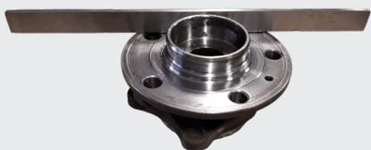
Check the surface for unevenness using a straightedge.
