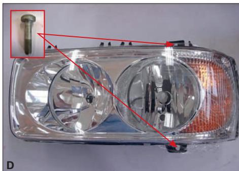
After assembling the lamp on the vehicle, lock the screw in the location (as shown on the right).
