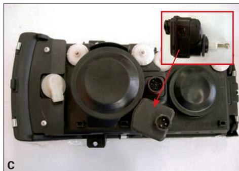
Install the servo motor in the original position. Please hook the reflector by hand. (Connect the bracket and reflector.)
