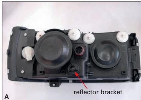
Rotate the reflector bracket to be loosened.
