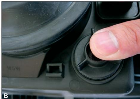
Take out the reflector bracket: Press the reflector bracket by hand. Then push it to loosen and remove at a slant.
