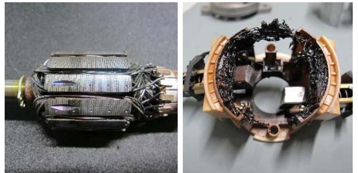
The photographs depict a disassembled secondary air pump with traces of overheating and melt marks.
