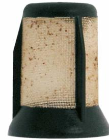
Prefilter of the E3T – blocked by rust
