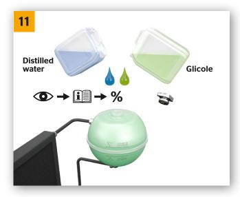
→ Fill cooling system with new coolant in correct mixing ratio of anti-freeze to water. Only use anti-freeze concentrates approved for vehicle. Different limit values (hardness, pH) apply to water used, depending on vehicle manufacturer and year of manufacture. If in doubt, use distilled water.
