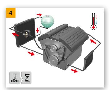
→ Bring engine to operating temperature so that coolant thermostat opens large cooling circuit. Switch heater to highest setting, leave to act for period specified in manufacturer's specification for product.
