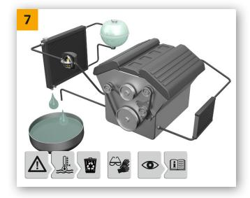
→ Fill coolant circuit with clear water. Bring engine to operating temperature at 2500 rpm and drain water again as described in steps 1 and 5.
