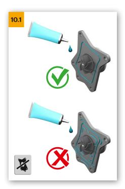
→ Fit new water pump in accordance with manufacturer's specification. It is essential to adhere to specified tightening torques and information on use of seals/sealants.
