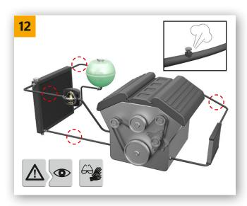
→ Bleed cooling circuit in accordance with manufacturer's specification (use filling device, if necessary) and check for leaks. Brief, slight escape of water at water pump drain opening is possible and will stop after short time.
