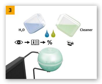
→ Mix clear water with cleaning additive (e.g. MB A0009891025, Liqui Moly 3320, etc.) in correct ratio and pour into cooling system.
