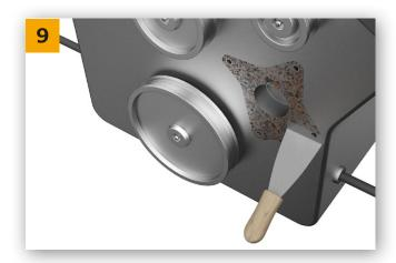
→ Now remove old water pump and thoroughly clean and degrease all seal surfaces.
