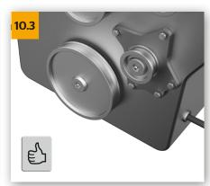
→ If water pump is prefitted with seal or O-ring, no sealant may be used. Wet prefitted O-rings with coolant before fitting pump. Do not use grease.
