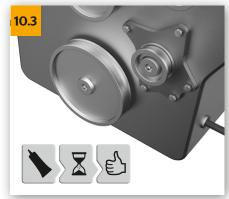
→ Only use sealing compound if this is explicitly specified for this water pump. In water pumps fitted using such a liquid sealant, ensure that sealant is applied sparingly and uniformly and that curing times are observed before refilling cooling circuit. Coolant can otherwise be contaminated. Tighten fastening bolts of water pump alternately to specified torque.
