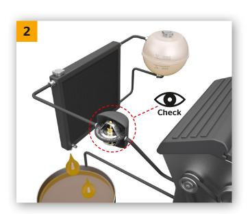
If old coolant is heavily contaminated, it is essential to check and, if necessary, replace thermostat.
