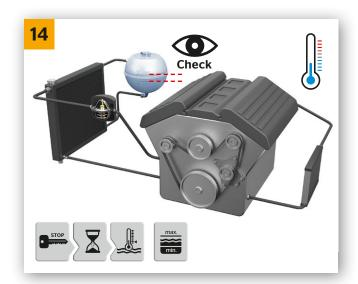
→ Carry out test drive or run until operating temperature has been reached. Then check again for leaks and system level (Caution: Risk of scalding).
