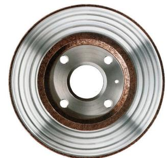
Corroded, cracked or worn disc; change in pairs
