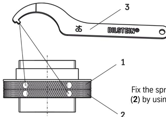
Fix the spring plate (1) and locknut (2) by using hook wrench (3) delivered by BILSTEIN.
