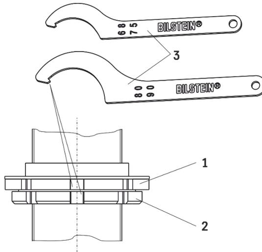
Fix the spring plate (1) and locknut (2) by using hook wrench (3) delivered by BILSTEIN.
