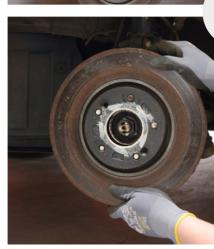
4. Remove the brake disc and check the brake components for damage, replacing them if necessary.
