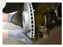
6. Now mount the new, perfectly fitting Herth+Buss brake disc onto the wheel hub. The new brake disc must be completely free of grease to ensure that the braking power is not compromised later on. Please note: it is not necessary to clean the brake disc or remove the coating before installation! After performing the repair, the vehicle should be braked hard four to five times from around 50 - 60 km/h during a test drive to remove the coating from the brake discs.
