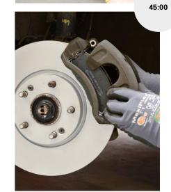
10. Now insert the new brake pads from the Jakoparts product range. The brake pads can be installed with the greatest of ease thanks to the assignment of preci-
