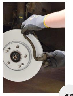
9. Apply a high-temperature-resistant, non-metallic permanent lubricant to the contact and guide surfaces of the brake calliper brackets and the brake pads.
