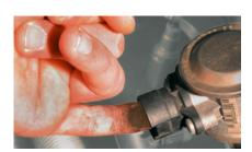
Finger test at secondary air valve in BMW 520i (highlighted)
