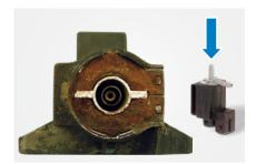
Corroded switchover valve (open)
