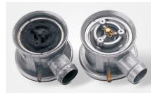
Open secondary air valve Left: Damage caused by exhaust gas condensate Right: New condition
