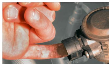
Finger test at secondary air valve in BMW 520i (highlighted)
