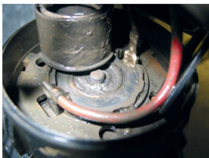
Corrosive exhaust gas condensate in the drive motor of a secondary-air pump
