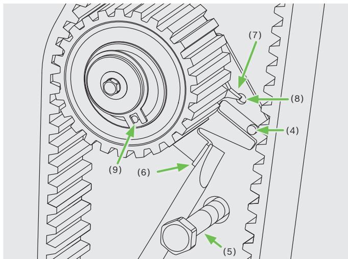
**Depending on the vehicle manufacturer and the model series, two different procedures are to be applied for the adjustment of the timing-belt tension.**
