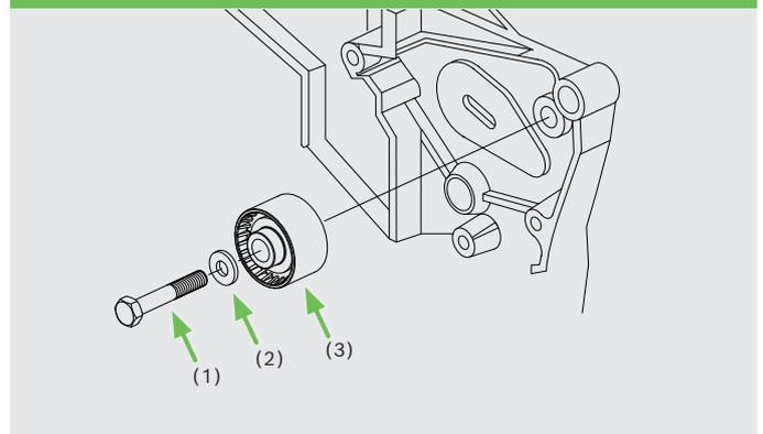
The idler pulley (3) is to be fitted together with the washer (2) and the bolt (1).
