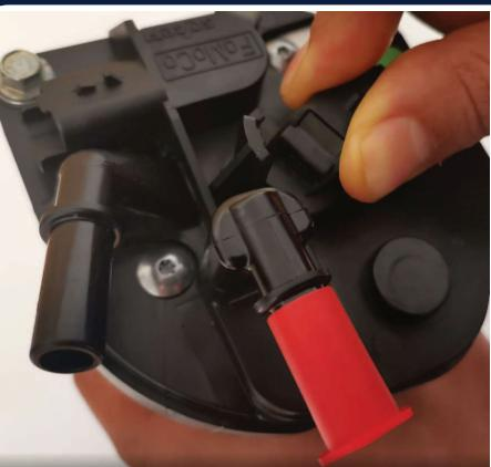
GB Push and turn the sensor, this time anti-clockwise, place it carefully in its seat and in the same axis. Finally put back the plastic support.
