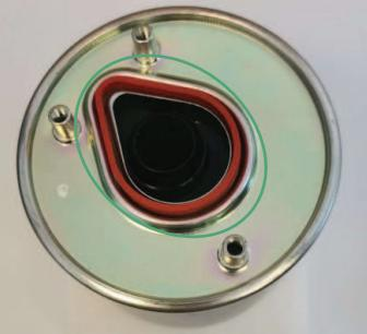
GB Lubricate and install the outer gasket in its place.
