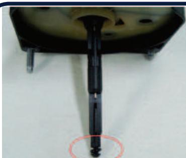
**(GB)** Check that the O-ring is not damaged.
