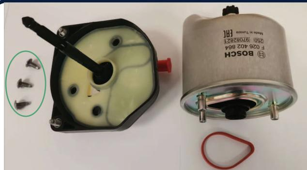
**(GB)** Remove the three screws from the plastic support and detach it from the filter.
