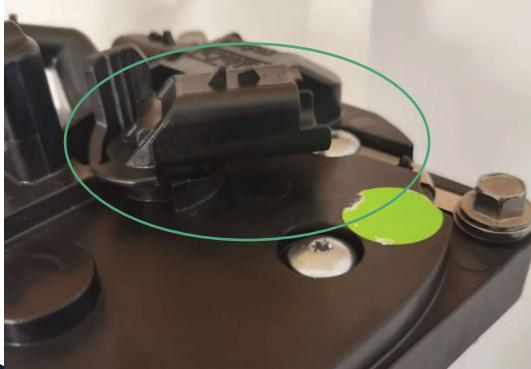
**(GB)** Turn clockwise the sensor and remove it from the filter element very carefully.
