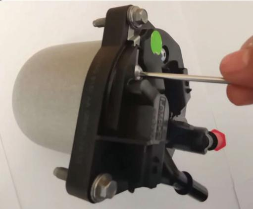
GB Tighten the three screws gradually going from one to other clockwise and repeat the operation until they are all tight.
