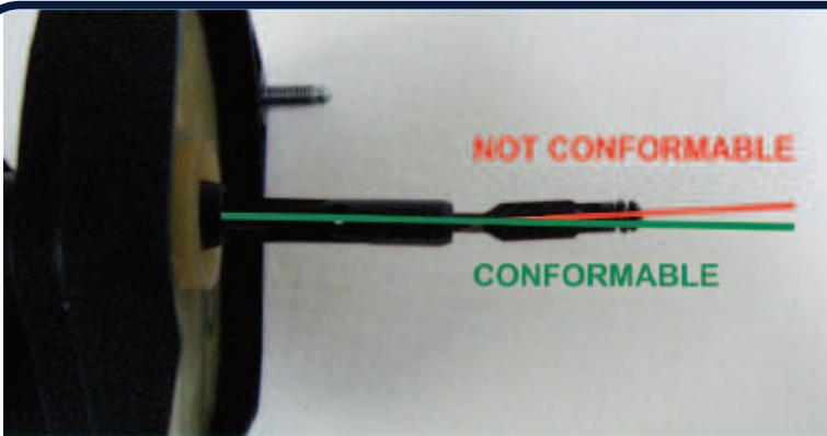
**(GB)** Make sure about the integrity and straight alignment of the sensor.
